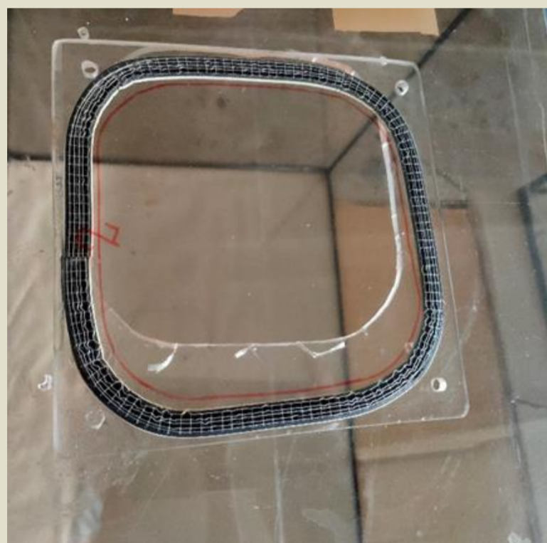
Fig. 1 Cover with gasket and fixing with screws
