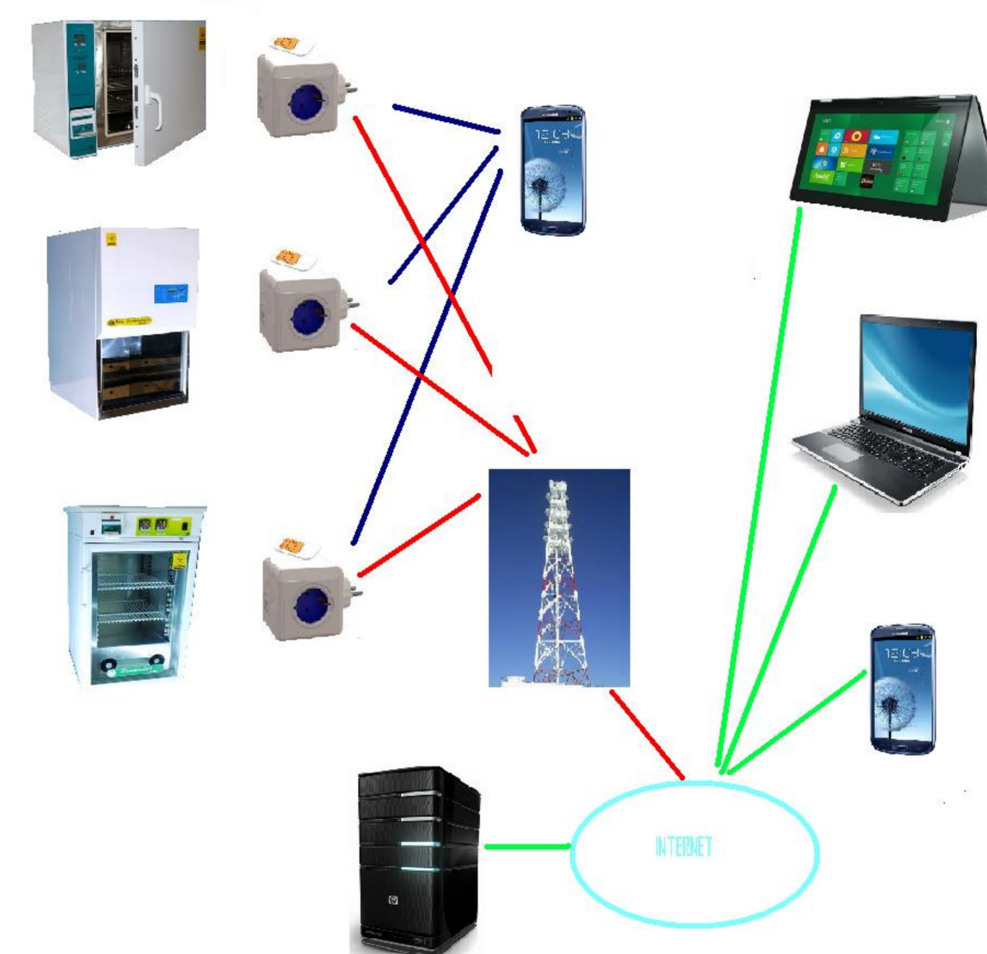
Fig. 1 Internet acquisition system for electromedical products
