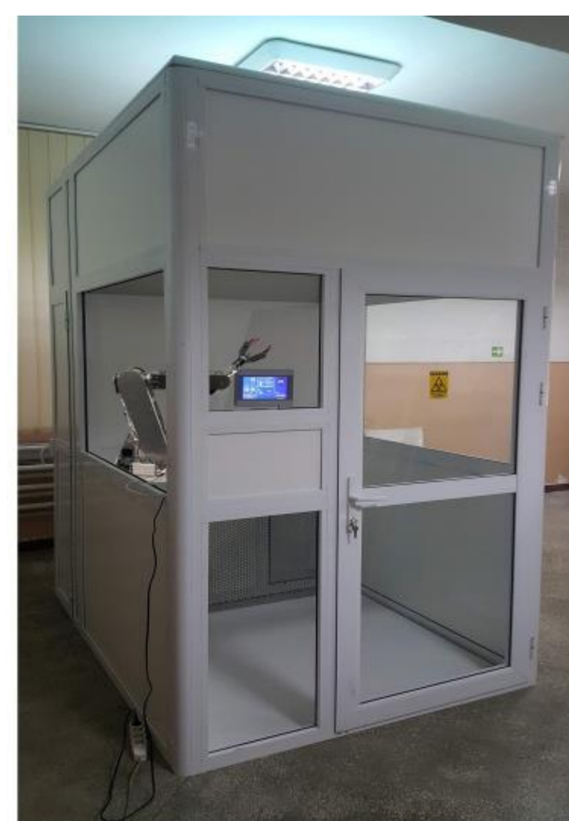
Figure 1. SAFE - Safety cabinet for collecting specimens contaminated with airborne pathogens
