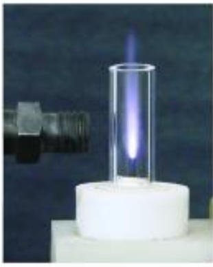
Figura 1. Photographs of: (a) miniaturized spectrometric equipment (assembly of components); (b) torch in which capacitively coupled, low power, low Air consumption microplasma is produced; (c) a passive sampling device based on the diffusion gradient in thin films technique
